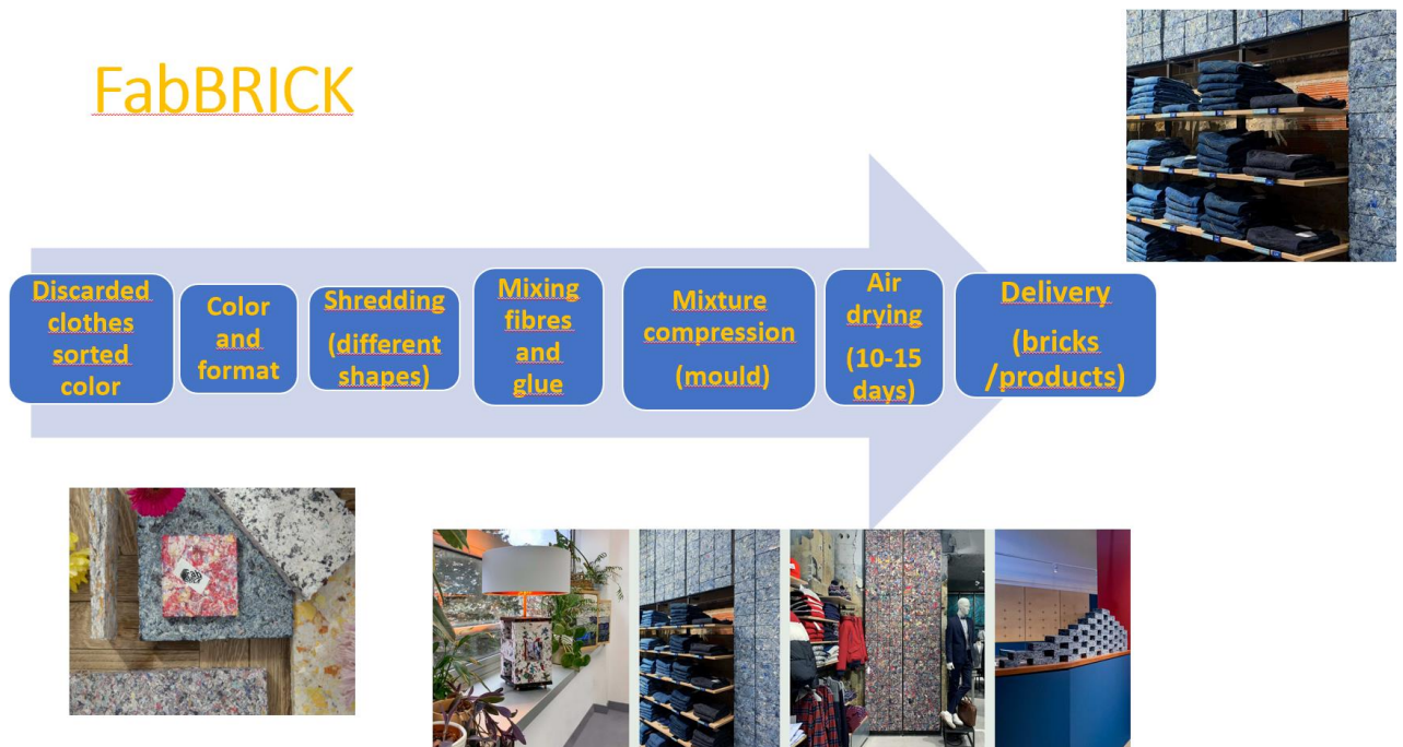
Fig. no. 27 Mechanical recycling by FabBRICK 80
